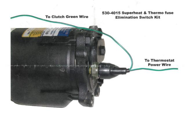
EVACUATE SYSTEM, REMOVE HPRV VALVE. INSTALL COPPER WASHER ON SWITCH AND INSTALL IN HPRV VALVE PORT (TORQUE 145 IN. LBS) CONNECT 1 WIRE OF PIG TAIL TO CLUTCH GREEN WIRE AND 1 WIRE TO THERMOSTAT POWER WIRE.
